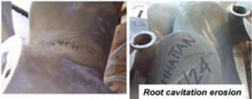
Root cavitation erosion
