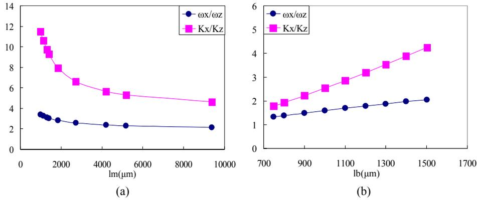
**Figure 4.** Resonance frequency ratio  $\omega_x/\omega_z$  and stiffness ratio  $K_x/K_z$  versus the length of seismic mass ( $l_m$ ) and the length of suspension beams ( $l_b$ )
