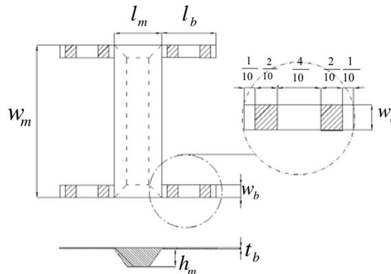
**Figure 1.** Schematic view of the piezoelectric micro-accelerometer
