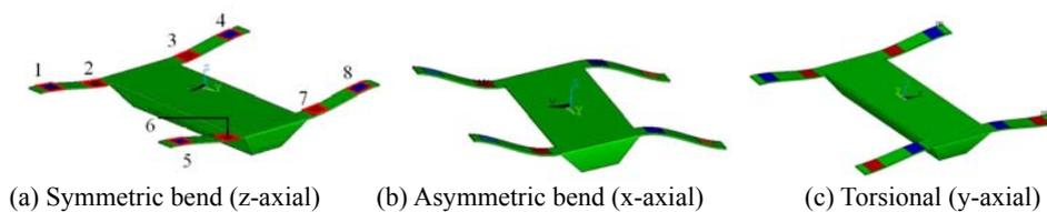
**Figure 2.** Three basic vibration modes of the accelerometer due to tri-axial acceleration
