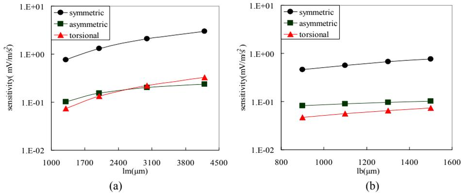
**Figure 5.** Sensor sensitivities versus the length of seismic mass ( $l_m$ ) and the length of suspension beams ( $l_b$ )
