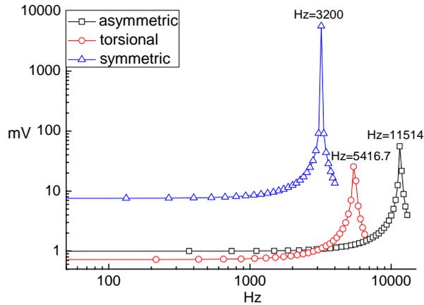
**Figure 3.** Frequency response of the accelerometer in triaxial acceleration
