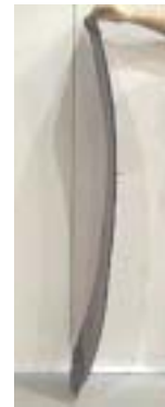
Figure 16. Example of part shape caused by a non-uniform cooling (warpage). This phenomenon is called banana effect at Lear Corporation.
