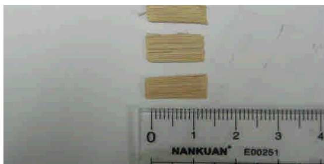
Figure 2. Bamboo fibers retain in sieve 4 with 13mm length.
