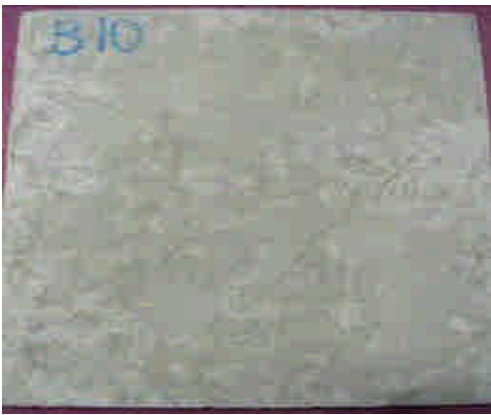
Figure 12. Reverse surface of B10 after incombustibility test.
