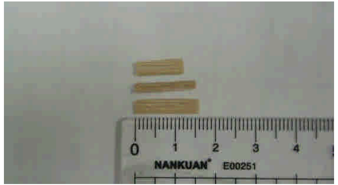
Figure 3. Bamboo fibers pass through sieve 4 and retain in sieve 8 with 15mm length.
