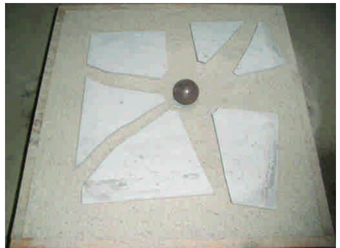
Figure 8. Fracture of counterpart material after impact test.
