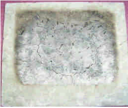
Figure 11. Heating surface of B10 after incombustibility test.
