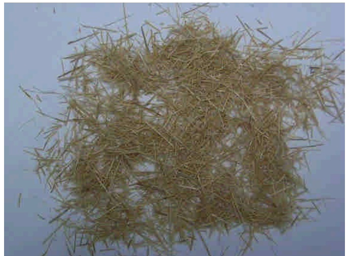
Figure 4. Bamboo fibers retain in sieve 50 with 5~15mm length.
