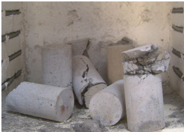
Fig. 1. RPC specimens spalled during ASTM standard fire test.
