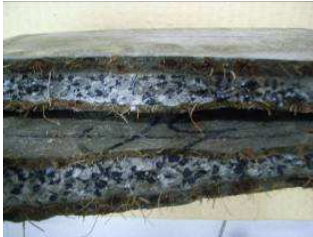
Fig. 5 Profile of bending breaking for LCRCB
