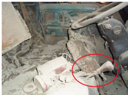
Figure 2. Truck inside tunnel with shifter at the top position.
