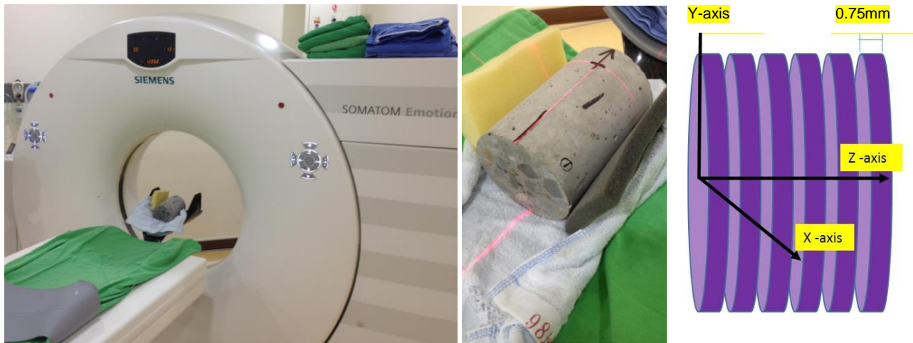
Figure 2. X-ray CT facility, the focus of the concrete cylinder while inserting for nondestructive CT scanning, and the orientation of the virtual segments (Photos taken by Dr. Yu-Min Su)
