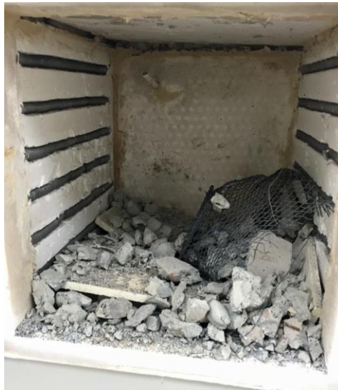
Figure 1. Shattered OPC concrete cylinder with broken protective steel meshes in the furnace (Photo taken by Dr. Yu-Min Su)
