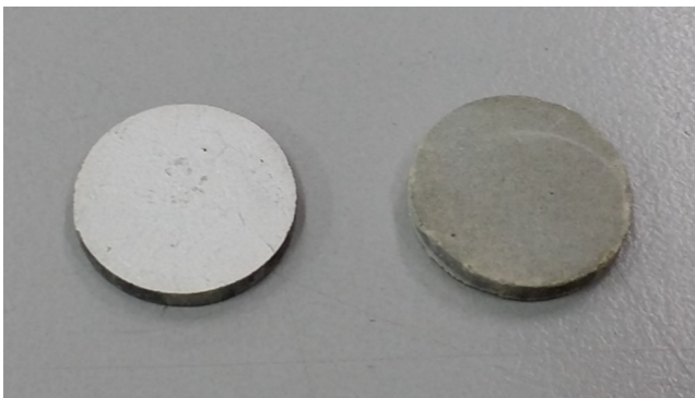
Fig. 2. The PZT/cement composite was coated with silver paint on the surface (left) to form the electrode and without silver paint coated (right).
