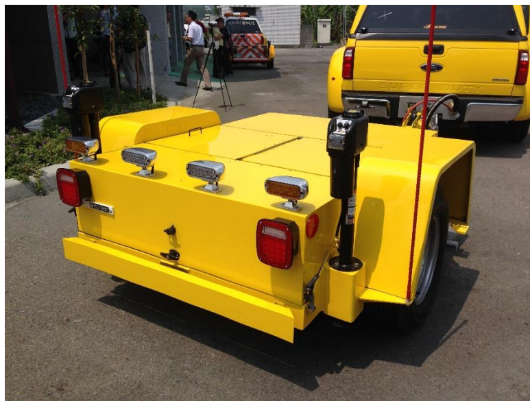
Figure 3: ASTM E-274 towed trailer of National Freeway Bureau in Taiwan. (Photo taken by Dr. Yu-Min Su)
