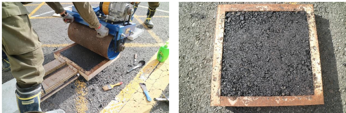
Figure 5: Compacting DGAC mixture into a wooden frame. (Photos taken by Mr. Siang-Hao Liang)
