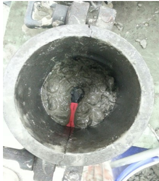
Figure 2. The piezoelectric sensor was placed in the middle of concrete cylinder
