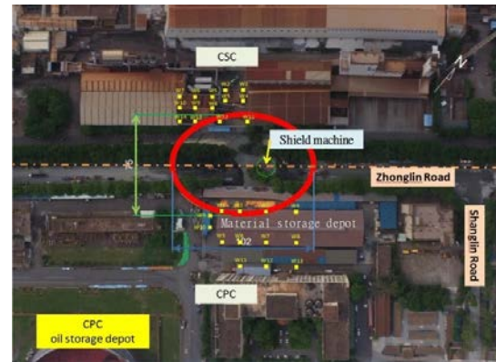
Figure 8. Hazard-impacted area and 36 monitoring points nearby, which include 14 points at the CSC warehouse and 22 points at the CPC warehouse.
