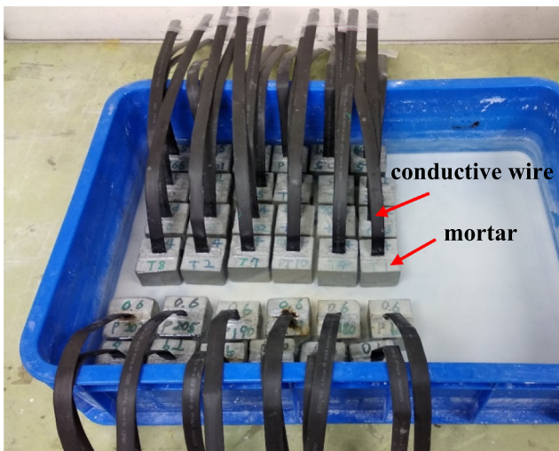
Fig. 5. Mortar specimens with embedded piezoelectric sensors cured in water.
