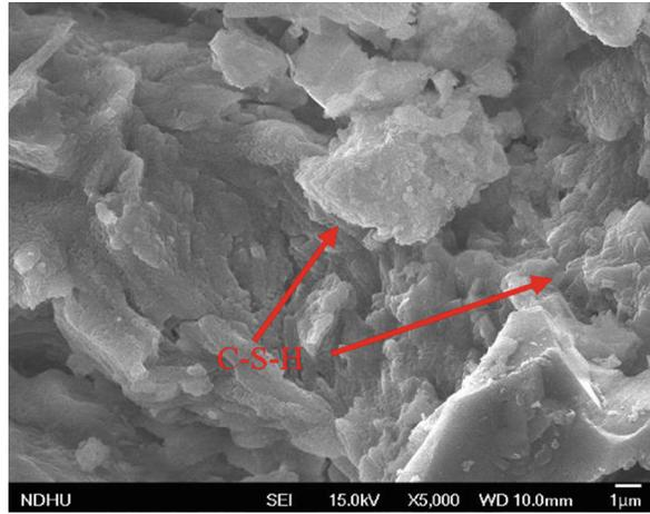
**Fig. 10** SEM photo for fly ash-precoated specimen
