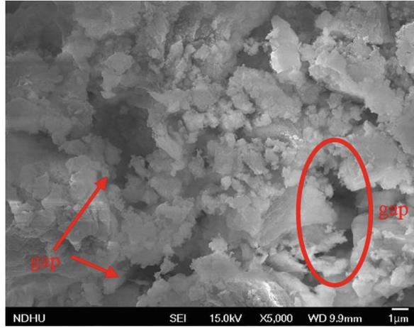
**Fig. 9** SEM photo for GGBS-precoated specimen
