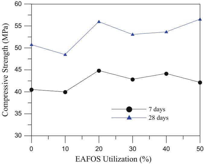
**Fig. 4** Development of EAFOS utilization against compressive strengths (GGBS-precoated)
