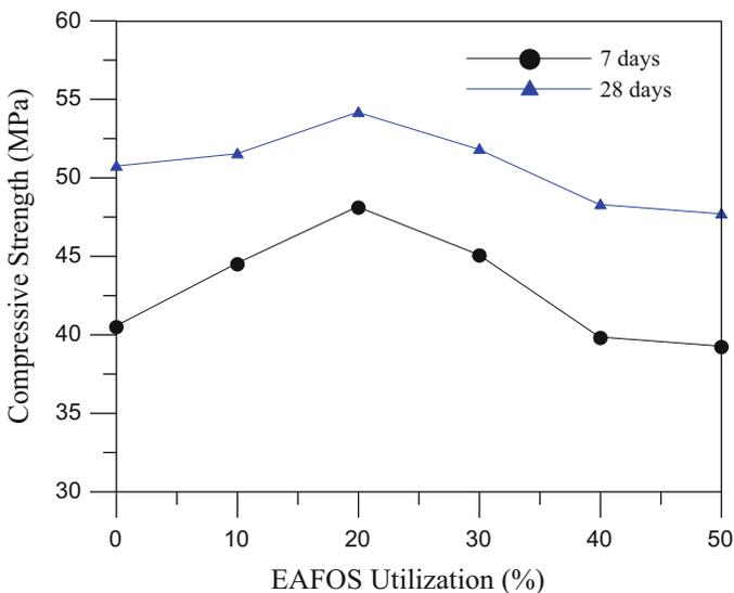
Fig. 3 Development of EAFOS utilization against compressive strengths (cement-precoated)
