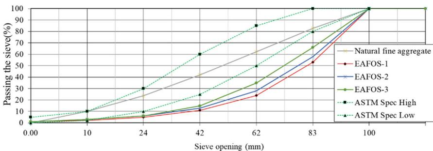
Fig. 1 Results of the EAFOS sieve analysis tests
