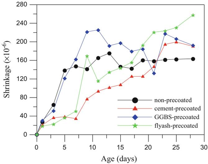
Fig. 6 Length variations of mortar specimens with different precoated methods
