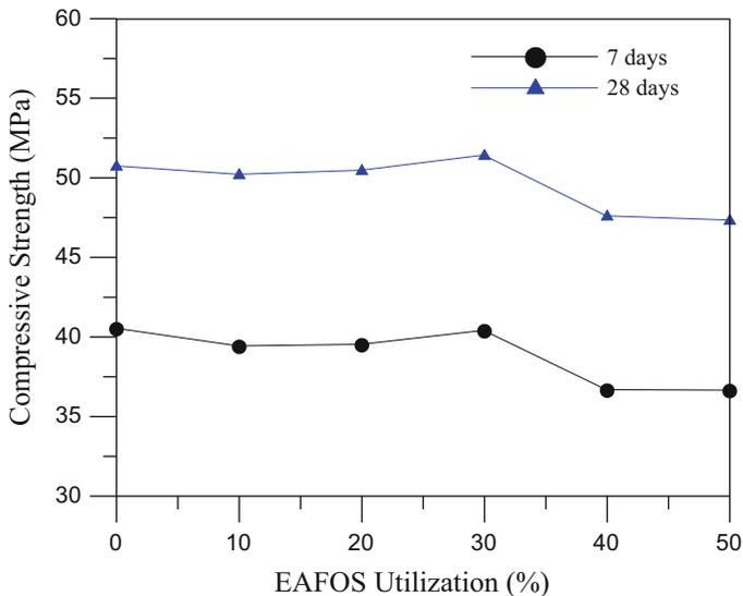
Fig. 2 Development of EAFOS utilization against compressive strengths (non-precoated)
