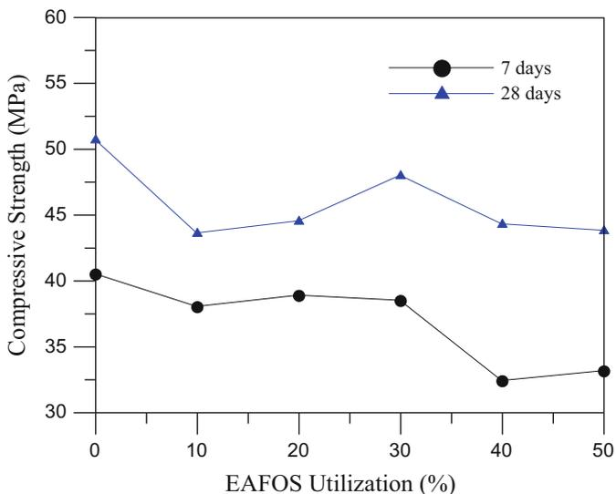
**Fig. 5** Development of EAFOS utilization against compressive strengths (fly ash-precoated)
